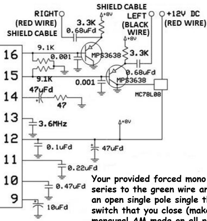
Your provided forced mono switch is wired in series to the green wire and +8V pad. This is an open single pole single throw (SPST) toggle switch that you close (make contact) to force monaural AM mode on all received stations.
